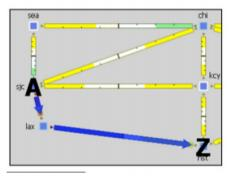
Bandwidth Optimization: Segment routing traffic engineering can find best path to meet bandwidth requirements
